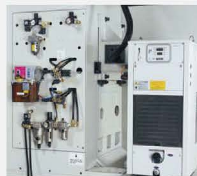
CONVENIENT AIR AND LUBRICATION SYSTEM MAINTENANCE The air lubrication systems are centralized at the back of the machine for convenient maintenance and inspection.
