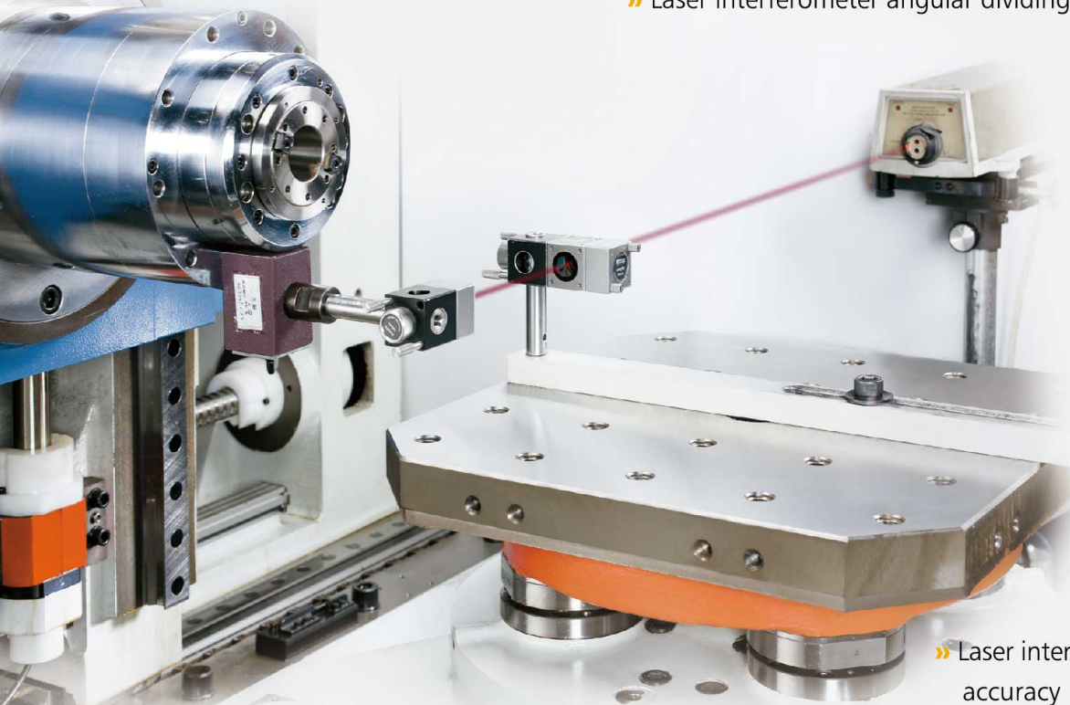
» Laser interferometer angular dividing accuracy measurement.
