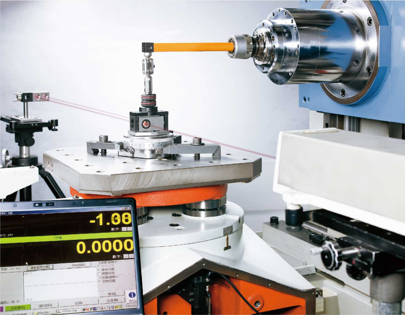
» Laser interferometer angular dividing accuracy measurement.
