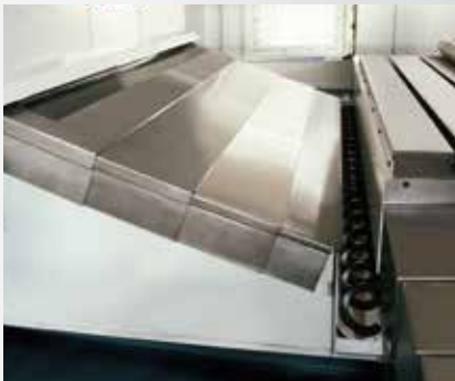
CHIP AUGER During machining, chips are flushed and fall down to the chip auger for delivering to the chip conveyor. It efficiently removes chips to eliminate being affected by chip heat and keeps work area clean at all times.
