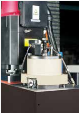
TOOL KNOCKING DEVICE »The tool knocking device with floating design features a buffering function which not only fully avoids damage to the spindle and bearings during tool release, but it also extends the service life of the spindle. »Tool knocking motion is actuated by an air cylinder for efficient tool release.
