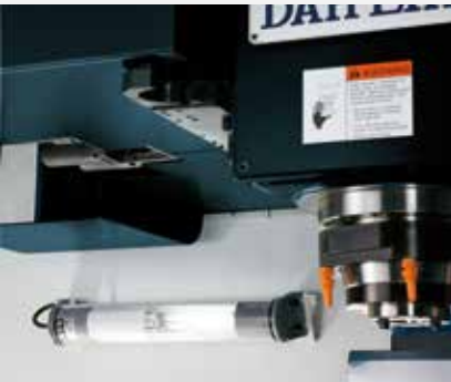
WORK LIGHT Two quartz work lights provide lighting for the working area. They feature soft illumination without being irritating to the operator's eyes.
