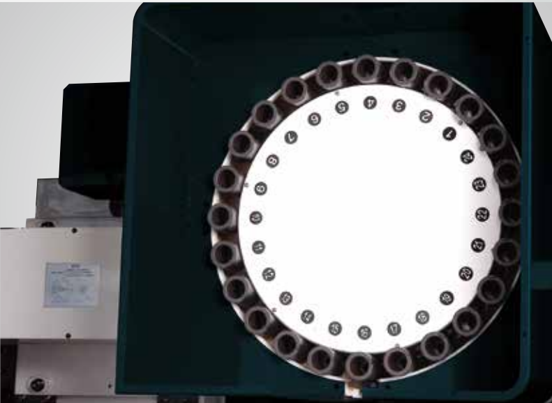
CAM TYPE MAGAZINE » The CAM type magazine rotation is driven by a cylindrical cam for fast and dependable tool change. Tool loading capacity is 30 tools. Random tool selection provides highly efficient tool changing.
