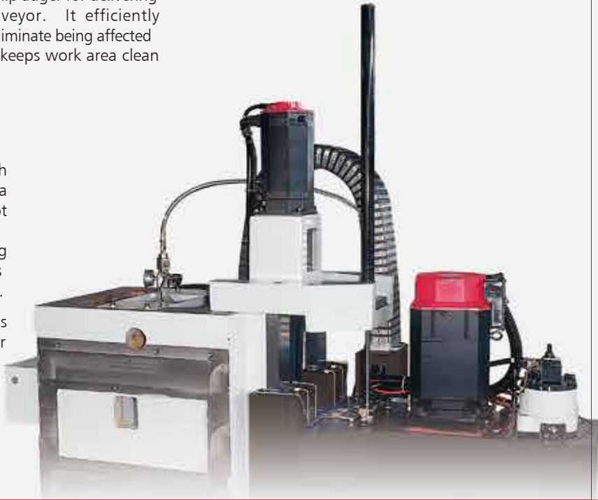
NITROGEN GAS COUNTER-BALANCE » The newly designed nitrogen gas counter-balancing system employs an accumulator which does not require additional power. » No hydraulic power unit is required. » No noise, extremely stable motion, no resonance and greatly upgrades machining efficiency. » Easy to adjust servo parameters.
