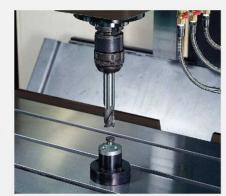
**AUTOMATIC TOOL LENGTH** MEASURING DEVICE (DAHLIH)
